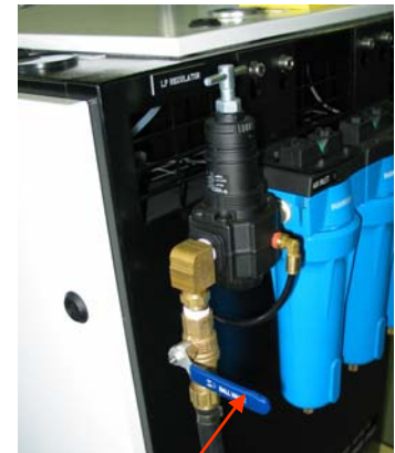
On/Off Flow Valve Handle in Off Position
